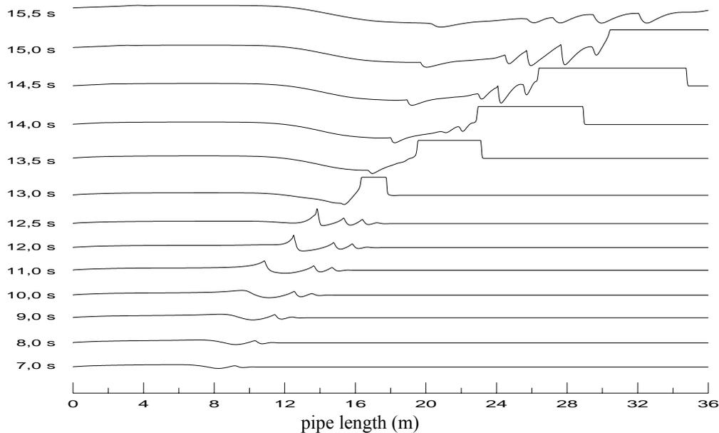
Figure 6. Liquid *holdup* distribution along the pipe for different time instants.  $U_{s_g} = 6.0$  m/s e  $U_{s_l} = 0.4$  m/s.
