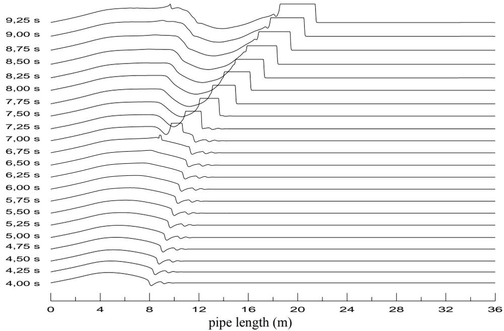
Figure 4 - Liquid *holdup* distribution along the pipe for different time instants.  $U_{s_g} = 2.0$  m/s e  $U_{s_l} = 1.0$  m/s.
