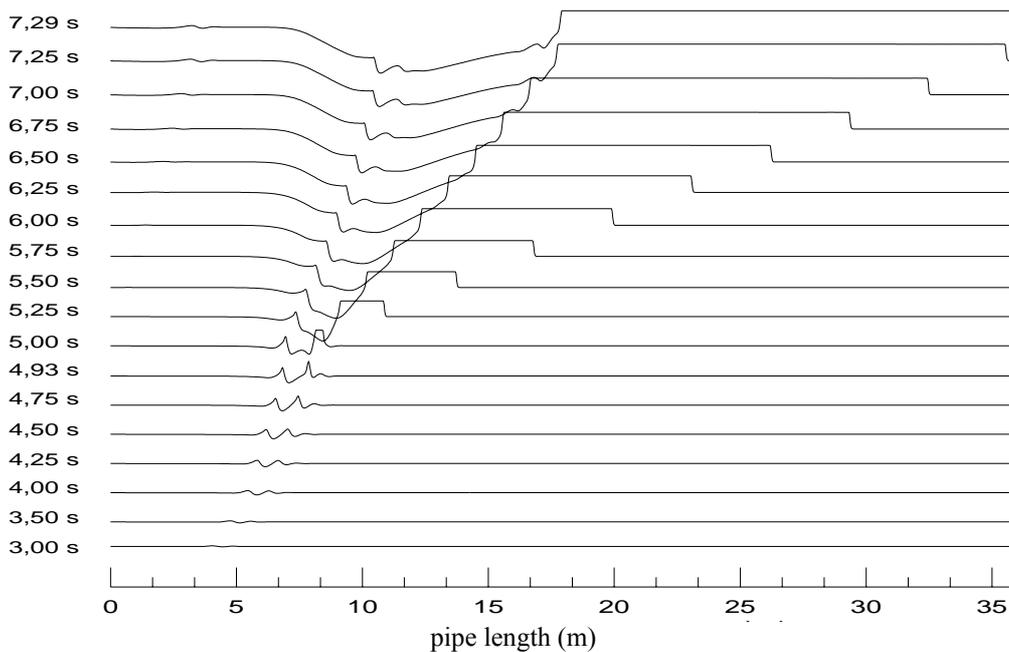
Figure 5. Liquid *holdup* distribution along the pipe for different time instants.  $U_{s_g} = 3.0$  m/s e  $U_{s_l} = 0.55$  m/s.
