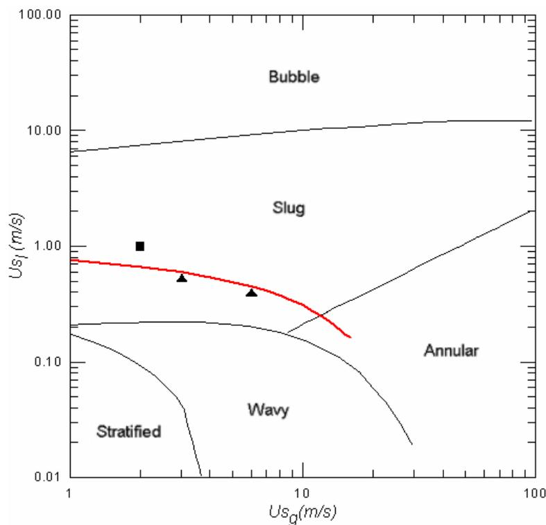
Figure 3. Flow pattern map of Taitel & Dukler (1976). Location of test cases on the map.
