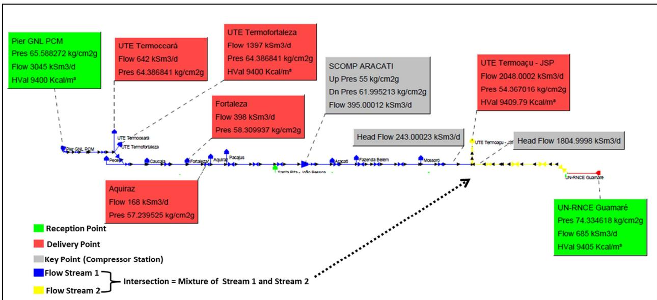
Figure 5 – Real Simulation Result in PLS
