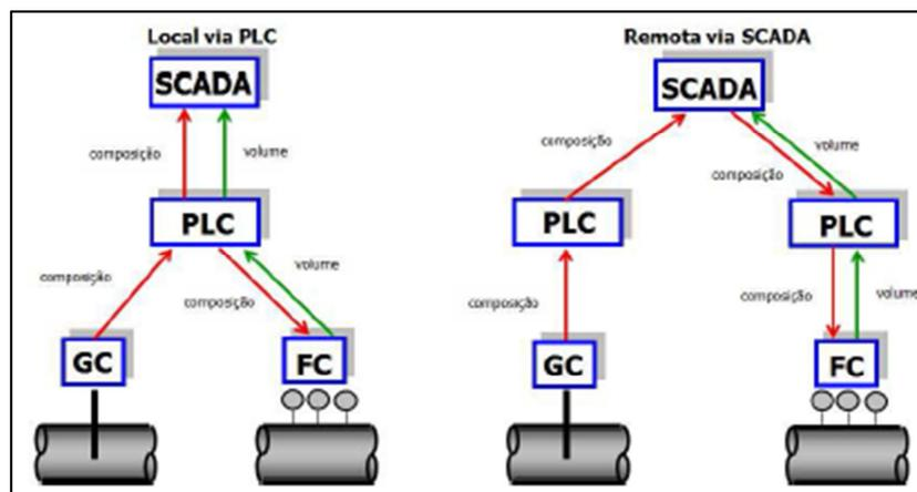
Figure 1 – Modes of writing chromatography on flow computers – on the left, one single station, with a Flow Computer and a Gas Chromatograph; on the right, two stations, one with the Flow Computer, and the other with the Gas Chromatograph.
