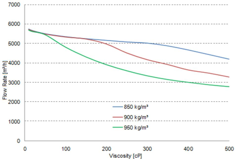
Figure 8. Flow Rate x Viscosity for the VISC 42 Pipeline
