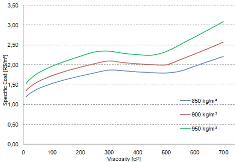
Figure 7. Specific Cost x Viscosity for the VISC 30 Pipeline
