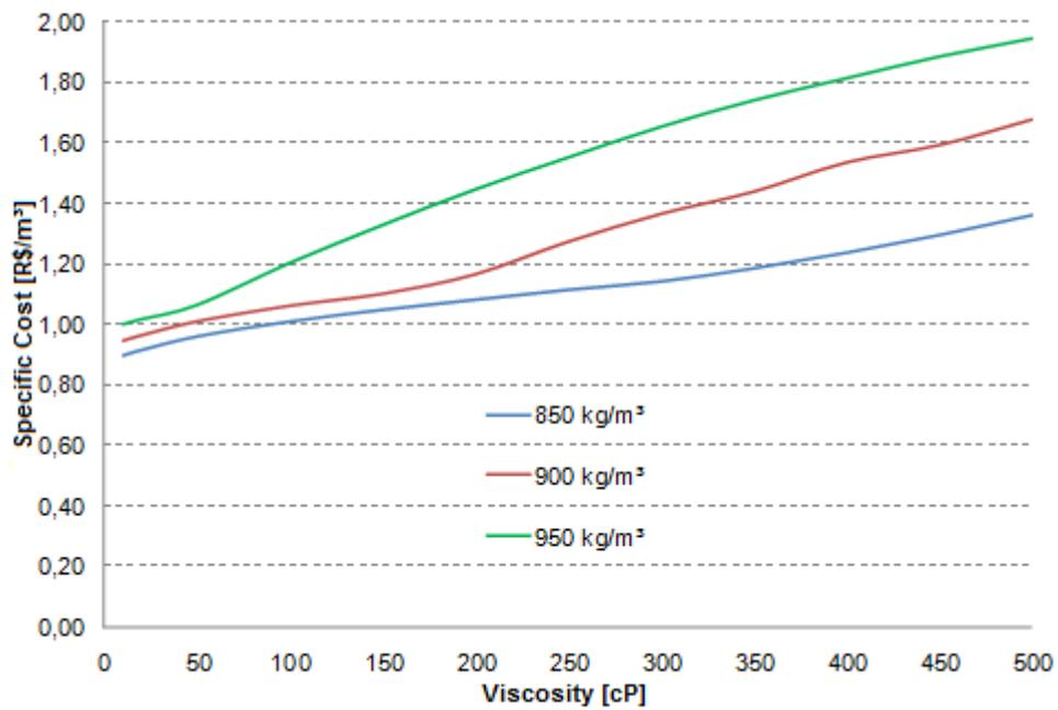
Figure 9. Specific Cost x Viscosity for the VISC 42 Pipeline
