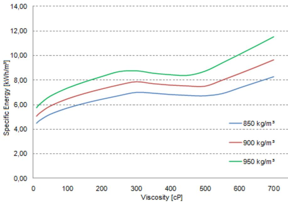
Figure 6. Specific Energy x Viscosity for the VISC 30 Pipeline
