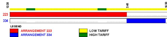
Figure 8: Optimal distribution of pumping arrangements – Case Study 2
