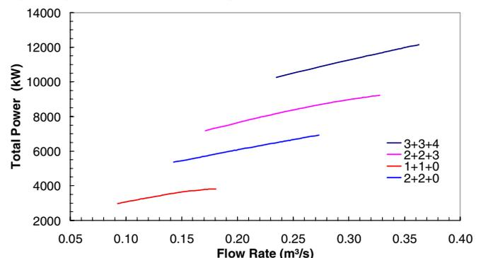
Figure 3 – Total pumping power required as a function of flow rate.
