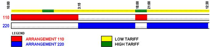
Figure 7: Optimal distribution of pumping arrangements – Case Study 1
